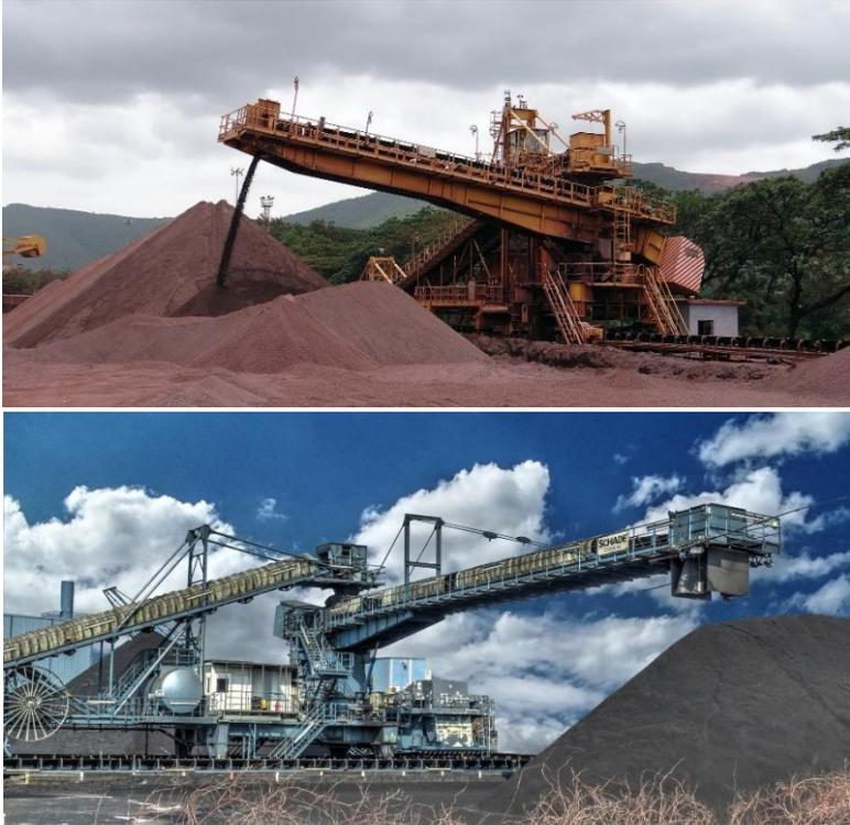
Gambar 8.14 *Stacker* Pada *Stockpile*
